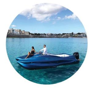
COULD THE Mambo represent the future of boat building? The wild-looking 21-footer, introduced during October's Genoa International Boat Show, was built by Moi Composites via its Continuous Fiber Manufacturing process, which uses a computer and 3-D printer to simultaneously build and shape a boat by adding individual layers of composite materials that are then cured by laser.
