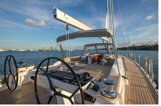
the deck. The windlass and chain locker are also under the deck. All halyards and control lines at the mast lead aft through under-deck conduits (each line has its own private tube) to the electric winches at the twin helms. Even the deck cleats are folding models that are stylish and unobtrusive.
