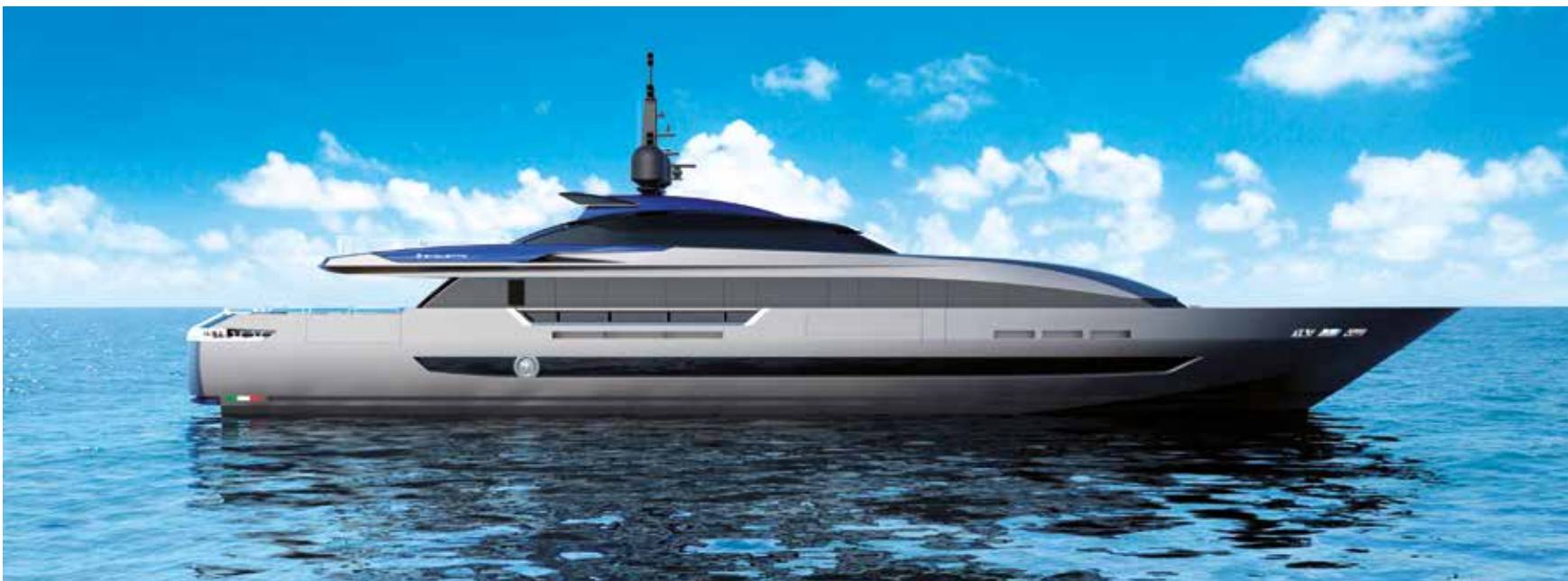
Above and below, one of the designs by Francesco Paszkowski (top, in frame) for Baglietto. The 43 Fast is a 43.65-metre all-aluminium planing yacht that promises a top speed of 30 knots. Its sporty exterior recalls elements of car design.
