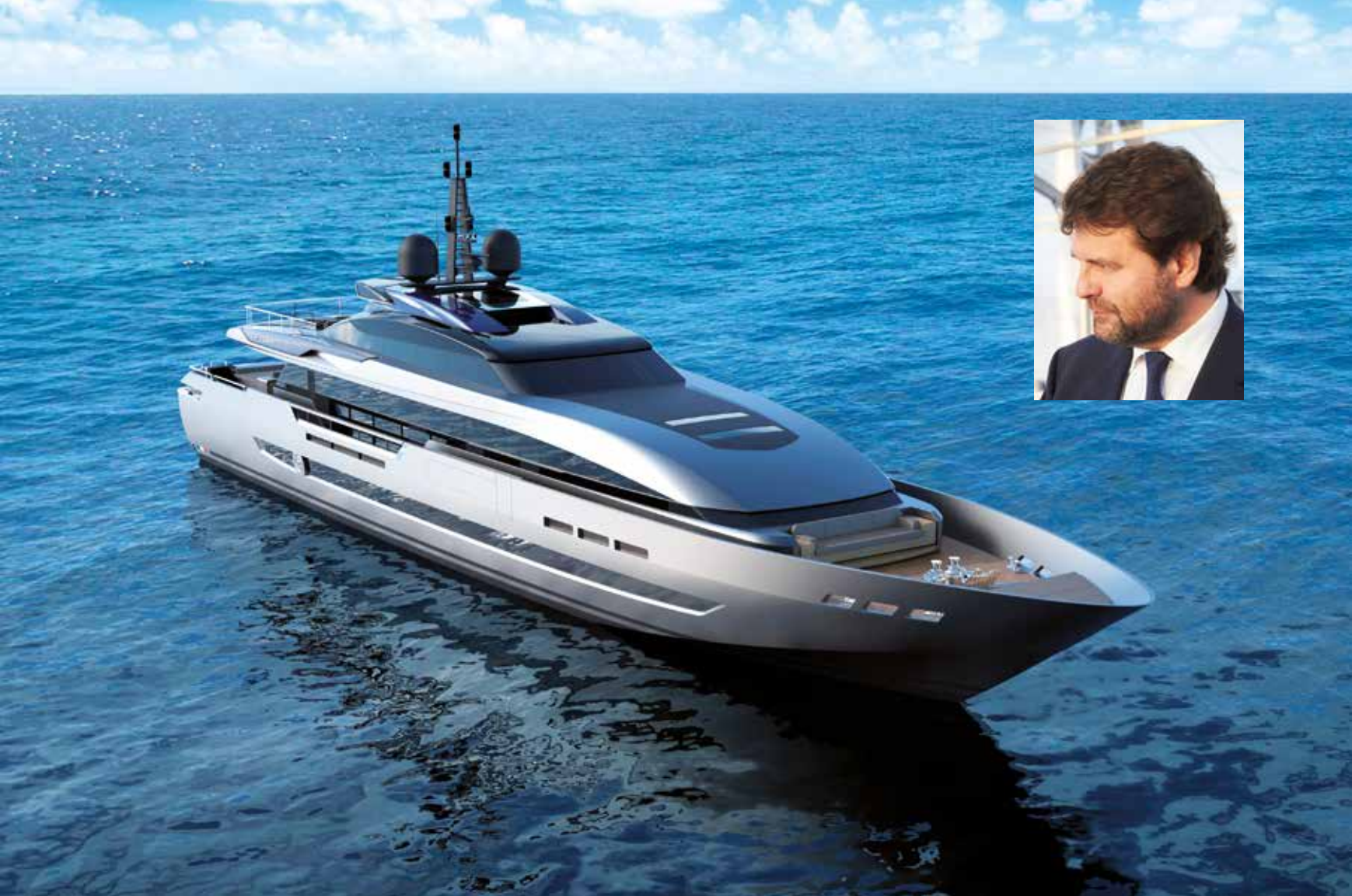
Above and below, one of the designs by Francesco Paszkowski (top, in frame) for Baglietto. The 43 Fast is a 43.65-metre all-aluminium planing yacht that promises a top speed of 30 knots. Its sporty exterior recalls elements of car design.
