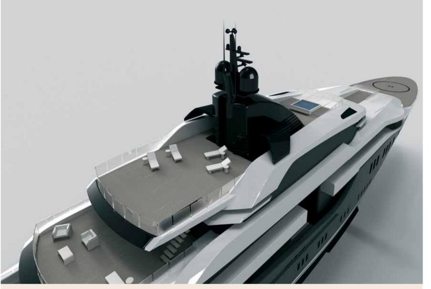
Forward on the Oceanco PA168, the super yacht's hull profile has a classic sloping The decks boast bow and a completely flat, clear fore deck, with a helipad platform that can be extended using the twin side extensions to allow large helicopters to land, in compliance with the new rules applicable to touch and go operations.
